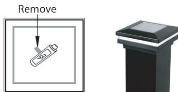
**Replacement Battery Specs:** IFR14500 (AA size), LiFePO4 3.2V, 600mAh or higher. Do not use regular/other batteries in the solar post cap light. The battery should last 3-5 years.
